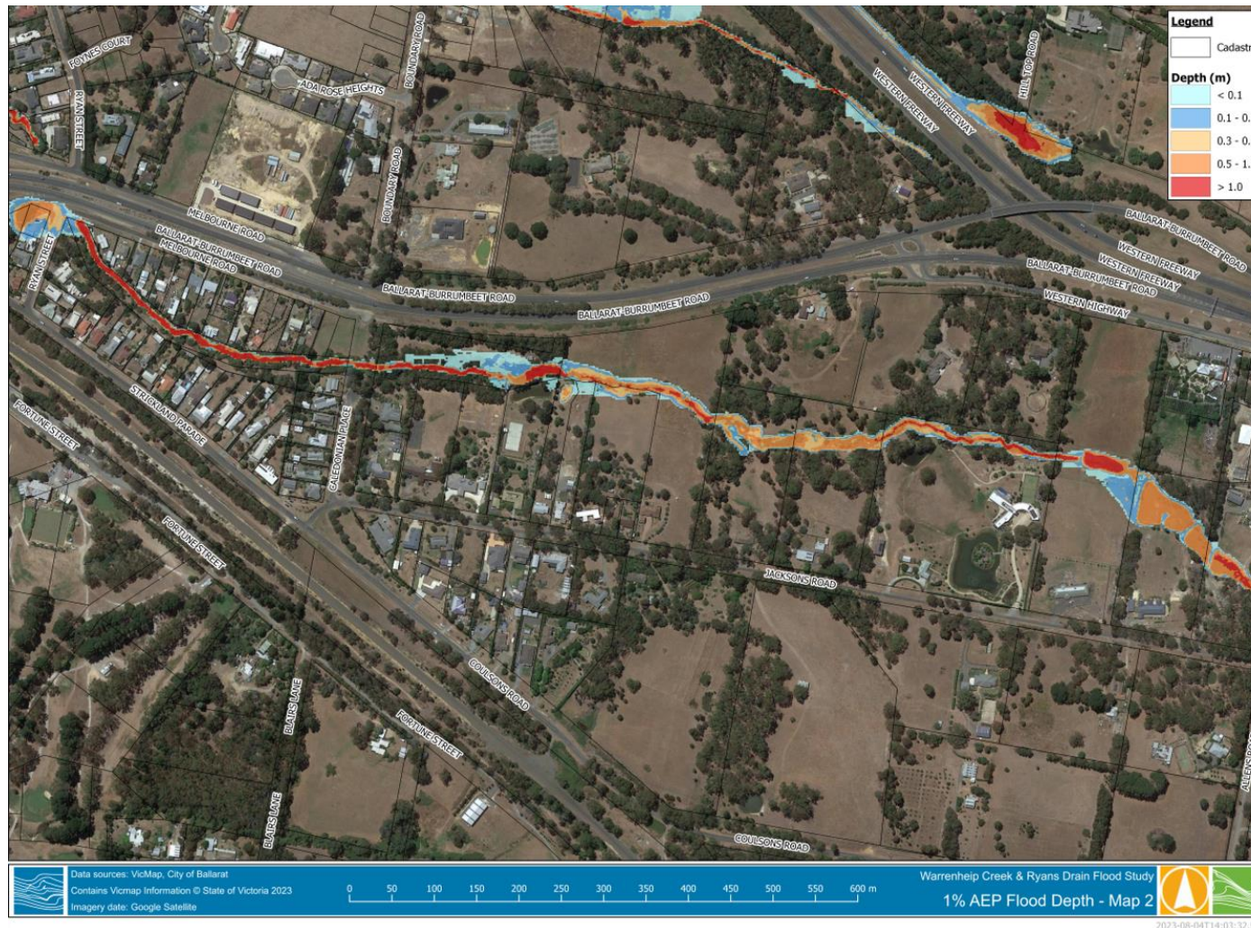
FIGURE 6-2 MAXIMUM FLOOD DEPTH – 1% AEP (VIEW 2)
