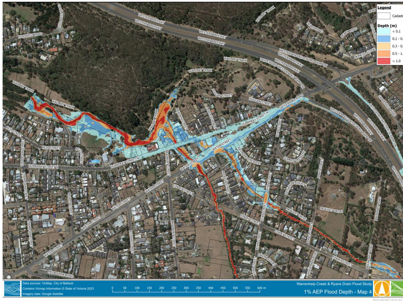
FIGURE 6-4 MAXIMUM FLOOD DEPTH – 1% AEP (VIEW 4)
