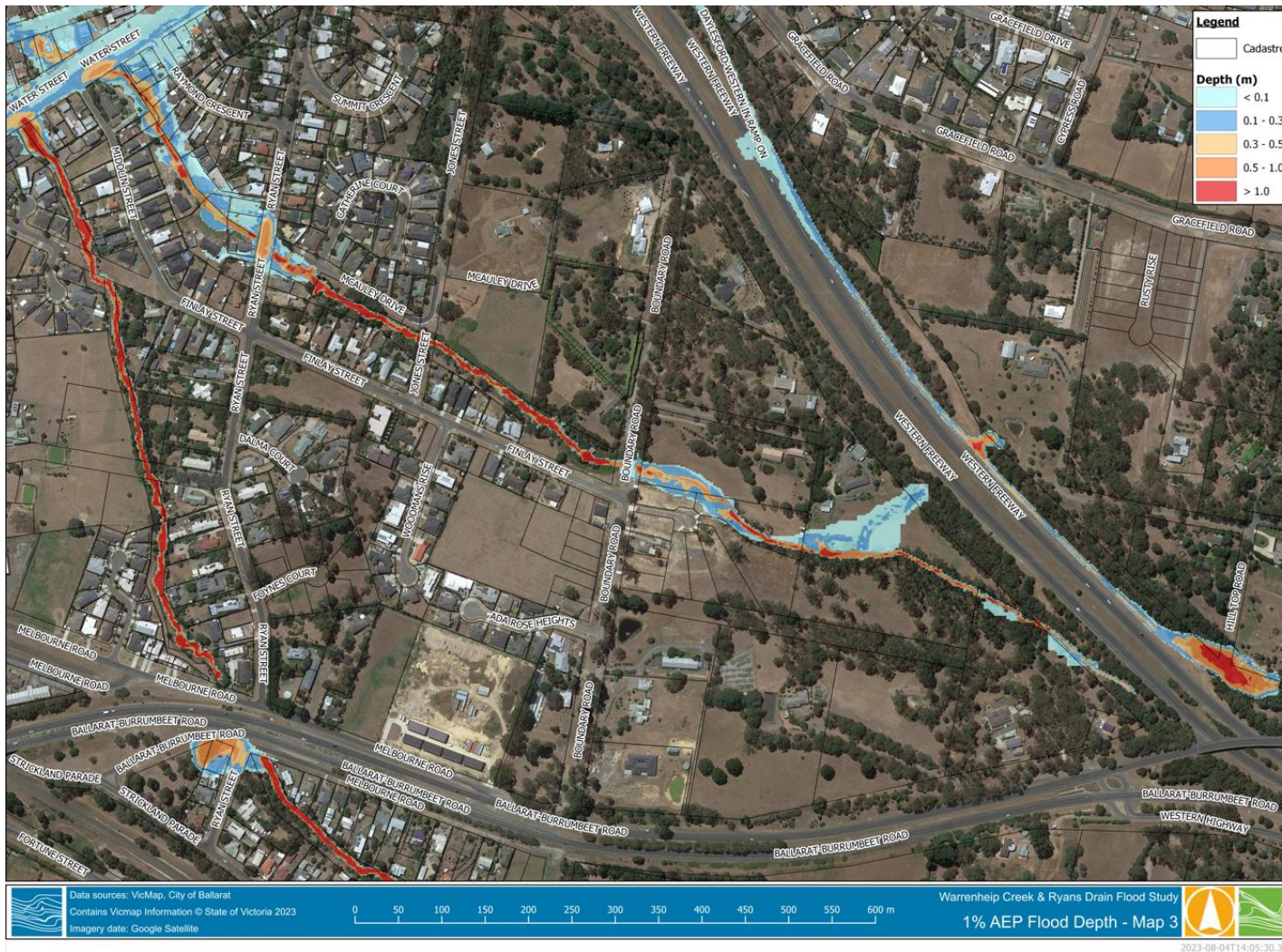
FIGURE 6-3 MAXIMUM FLOOD DEPTH – 1% AEP (VIEW 3)
