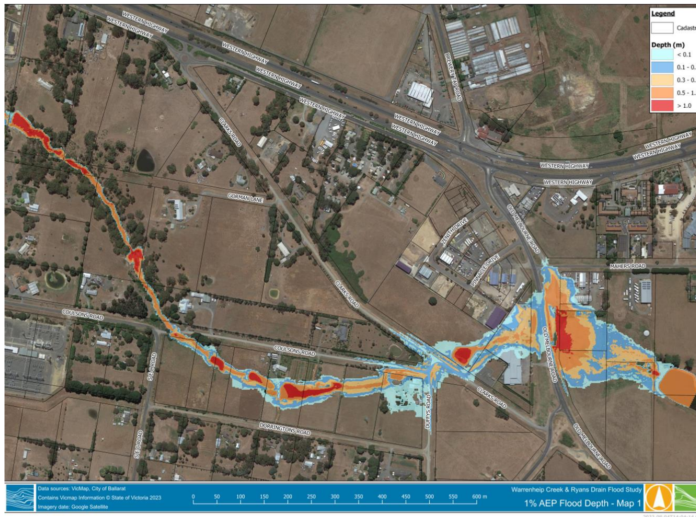
FIGURE 6-1 MAXIMUM FLOOD DEPTH – 1% AEP (VIEW 1)
