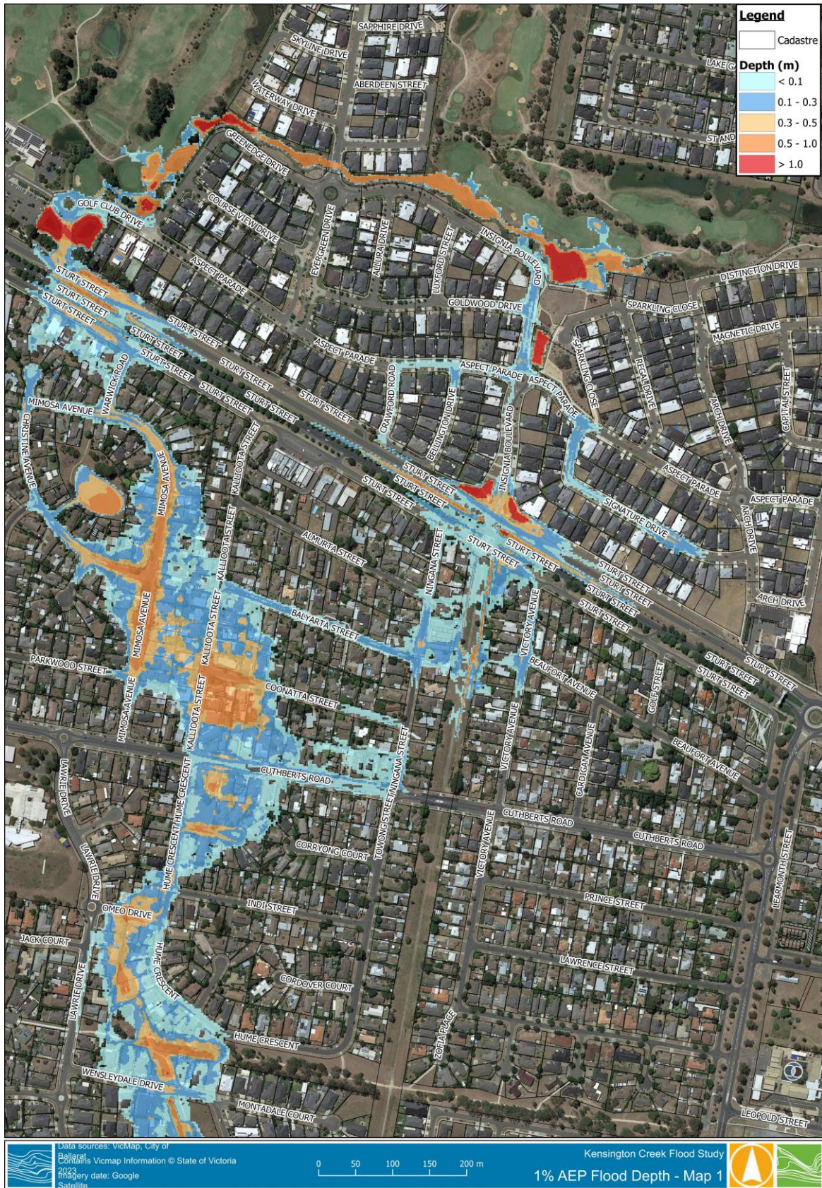
Figure 6-1 Kensington Creek 1% AEP Flood Depth – Map 1
