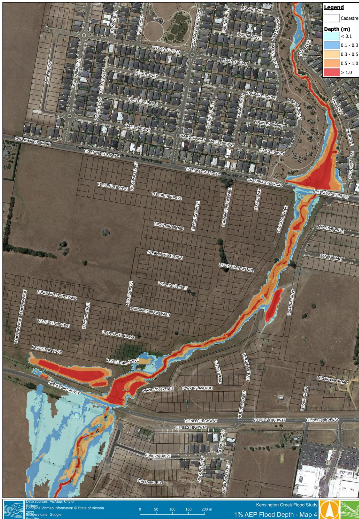
Figure 6-4 Kensington Creek 1% AEP Flood Depth – Map 4
