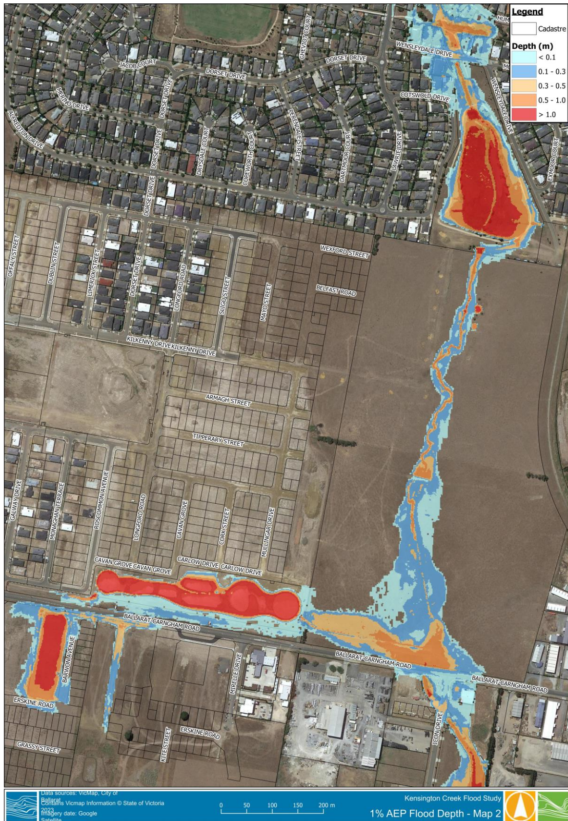
Figure 6-2 Kensington Creek 1% AEP Flood Depth – Map 2
