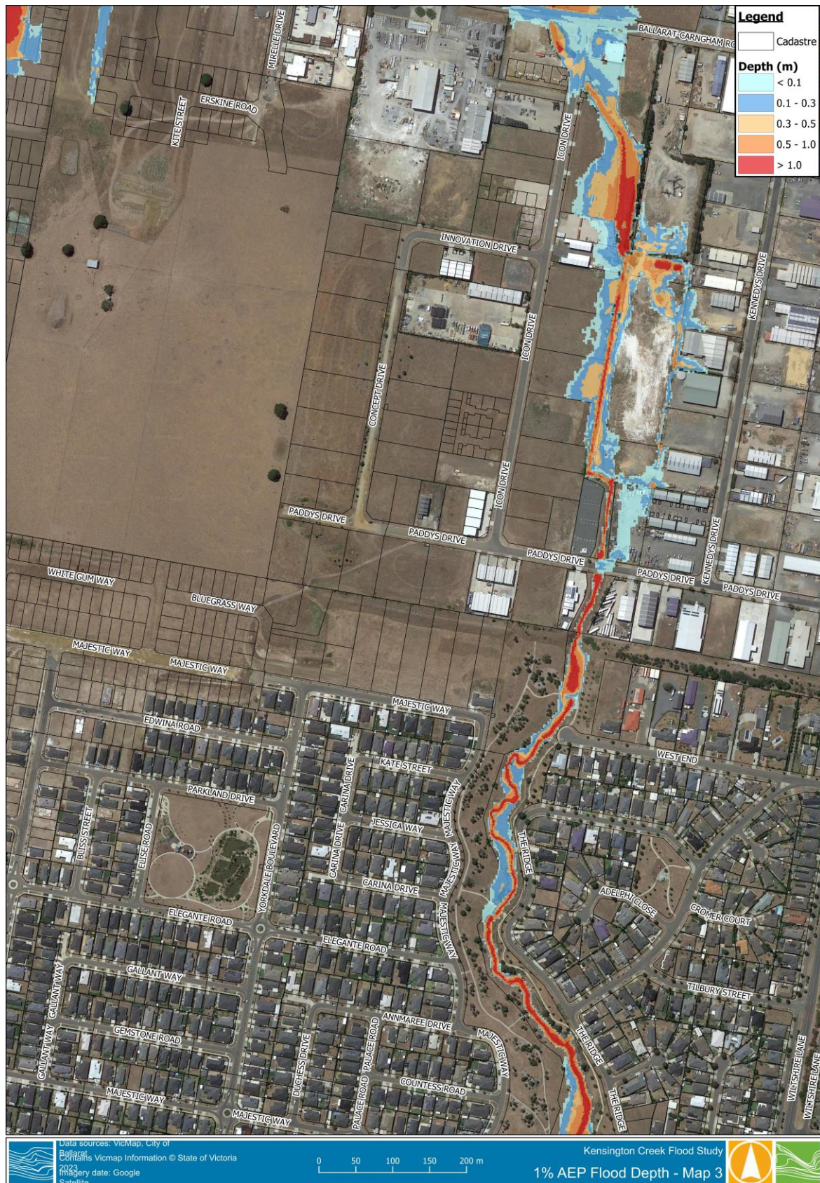
Figure 6-3 Kensington Creek 1% AEP Flood Depth – Map 3
